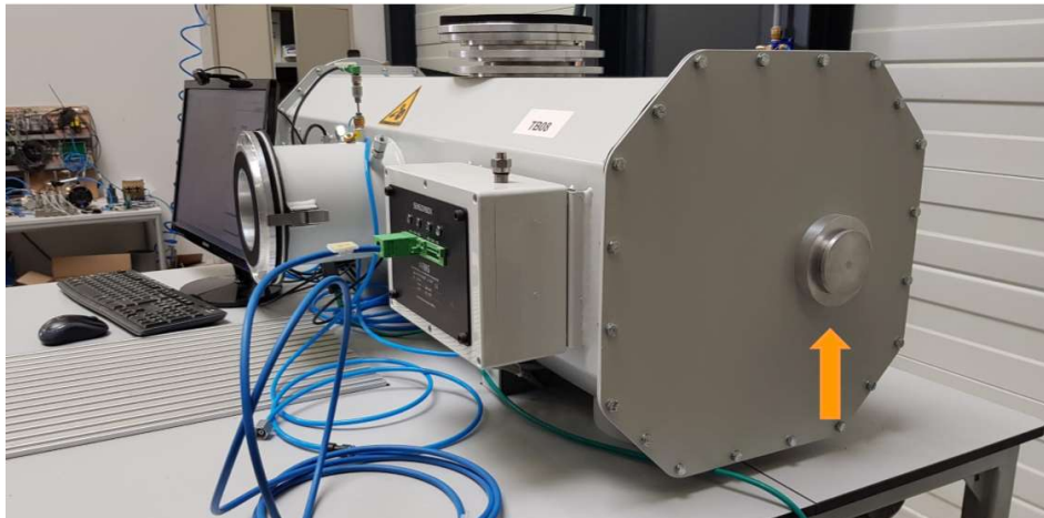
Image 3: 1.5" (DN40) to 6" (DN150) front side for testing RPD meters and turbine meters
